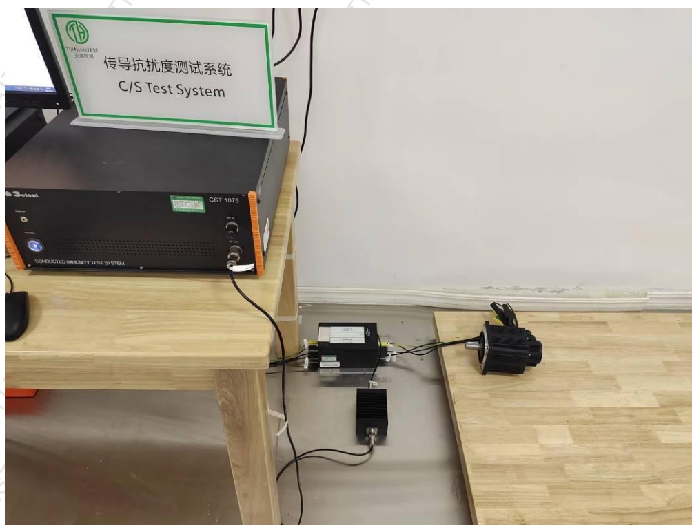
Photograph 7: Set-up for Conducted Susceptibility on AC Power and Signal Ports (CS)
