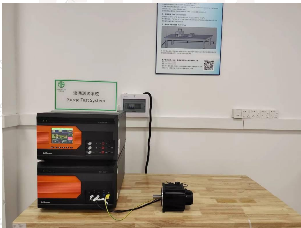
Photograph 6: Set-up for Surge on AC Power Ports
